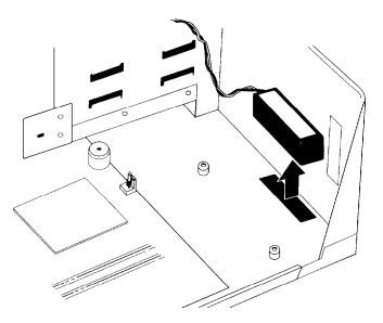
4. Remove the new battery from its package and position it so the Velcro faces down and the cable faces the power supply. Then push it down onto the bottom of the case.
